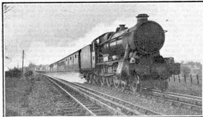
G.W.R. No. 1017 "County of Hereford," on a Birkenhead-Paddington express, taking water from Ruislip troughs. The engine is one of the new 4-6-0 "1000" Class. Photograph by C. R. L. Coles.
