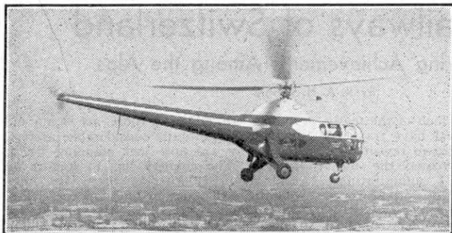
The long tapering fuselage of the Sikorsky S-51 commercial helicopter is well shown in this excellent flying view of the machine.
