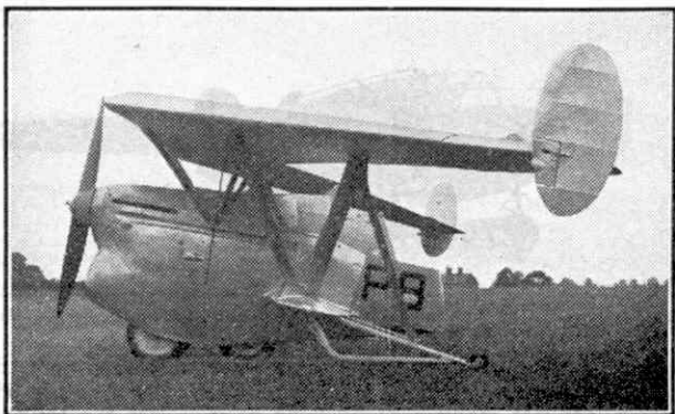
Westland "Pterodactyl," Mk. V two-seat biplane fighter. Photograph by courtesy of Westland Aircraft Ltd.
