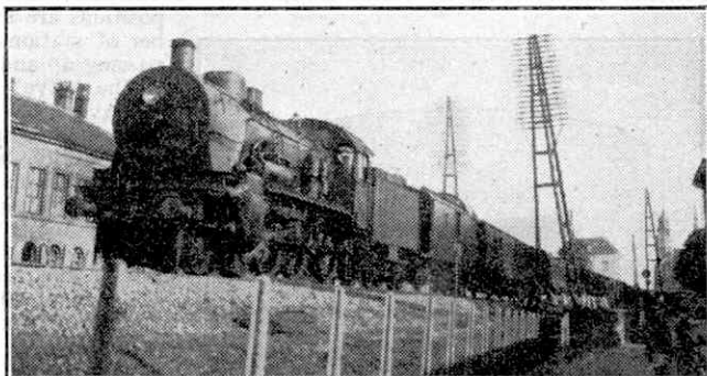
One of the numerous 4-6-0 locomotives of German origin of the Belgian State Railways. It is hauling a local train composed of typical Belgian stock used for secondary services.
