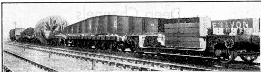
An outsize load by rail. A 130-ton stator that travelled by rail from Heaton, on Tyneside, to Birmingham. Photograph by courtesy of C. A. Parsons and Co. Ltd.
