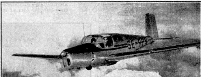
A new Swedish civil aircraft. The "Safir" is a 3-seater machine with a D.H. "Gipsy Major" engine. Photograph by courtesy of Svenska Aeroplan A.B.
