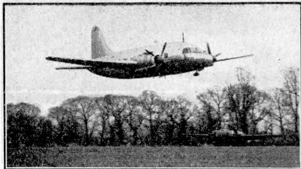
"Viking" transport demonstrating its ability to climb safely on one engine in the event of the other falling during take-off. Photograph by courtesy of Vickers-Armstrongs Ltd.
