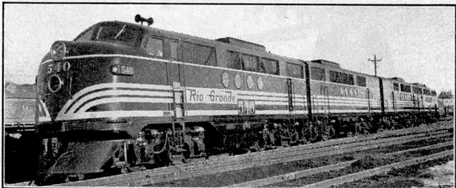
The shape of things to come in Britain? Denver and Rio Grande Western Railroad 5,400 h.p. 4-unit Diesel electric locomotive. Photograph by courtesy of the Denver and Rio Grande Western Railroad.
