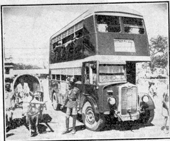
A typical traffic scene in Hyderabad, India, showing an Albion CX19 "Venturer" double decker bus owned by the Nizam of Hyderabad's State Railway, alongside a native bullock cart. Photograph by courtesy of C. C. Wakefield and Co. Ltd.
