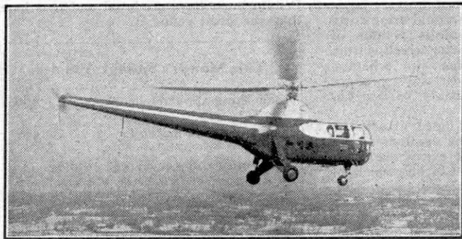
Sikorsky S-51 commercial helicopter, showing the long tapering fuselage. Photograph by courtesy of the United Aircraft Corporation, U.S.A.
