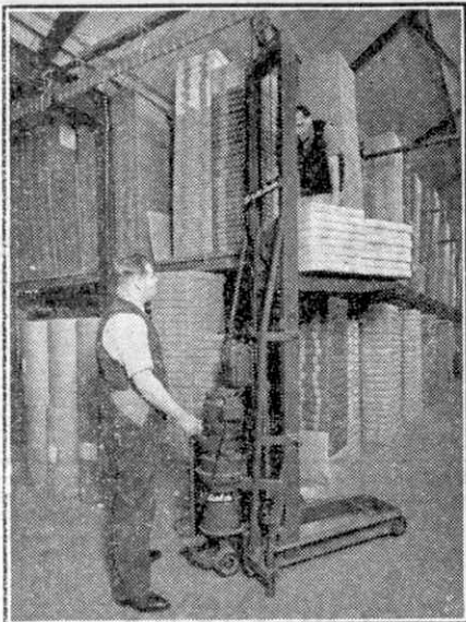
The Collis electric-hydraulic Stacker in use at a paper mill. This machine has a lift of 108 in. and a load capacity of 10 cwt.
