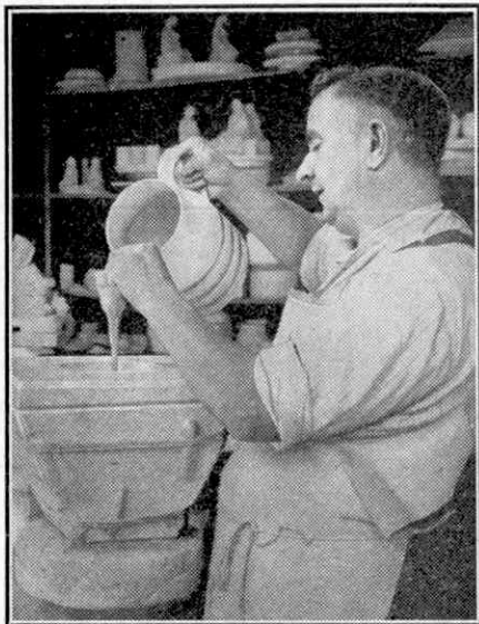
Pouring liquid clay (known as "slip") into the assembled moulds to form the cast model.
