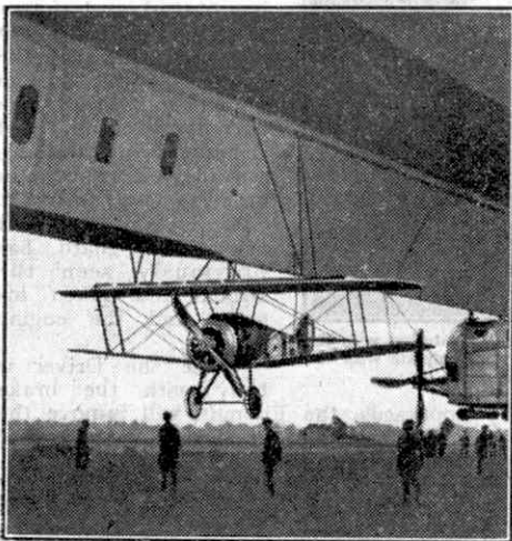
Sopwith "Camel" mounted under the British airship R23 at Howden in 1918. Photograph by courtesy of Imperial War Museum, London S.E.1.
