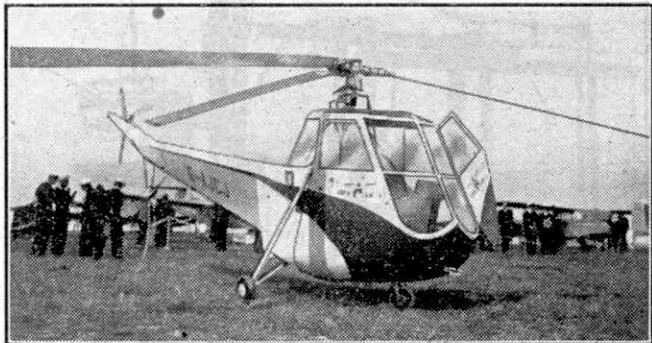
Cierva "Skeeter," a British two-seater light helicopter that loaded weighs only 1,200 lb. Further details are given above.
