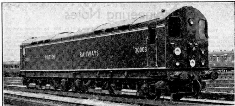
The latest Southern Electric locomotive No. 20003. It can work continuously for several days and nights and haul passenger trains at speeds up to 75 m.p.h., or 1,000 ton freight trains. British Railways Official Photograph.
