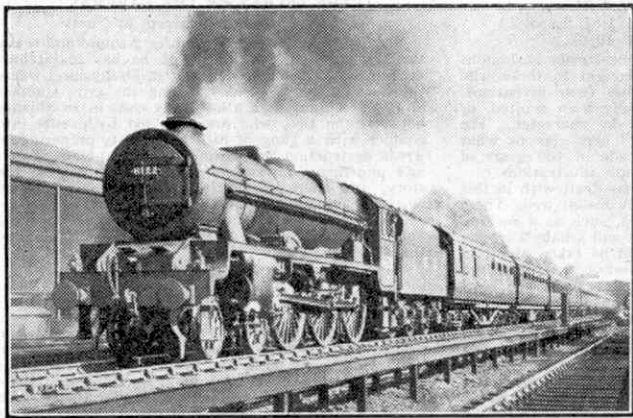
A Manchester express climbing Camden bank behind former L.M.S. 4-6-0 No. 6122 "Royal Ulster Rifles" of the converted "Royal Scot" Class. Photograph by F. R. Hebron.
