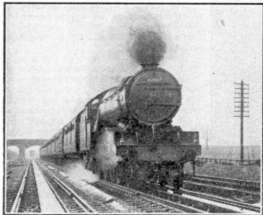
The new troughs in use at Wiske Moor. The engine of a down express picks up water.
