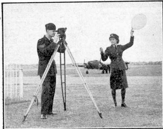
Ready to release a pilot balloon. When it is in the air sights are taken on it to find the speed and direction of the wind at various heights.
