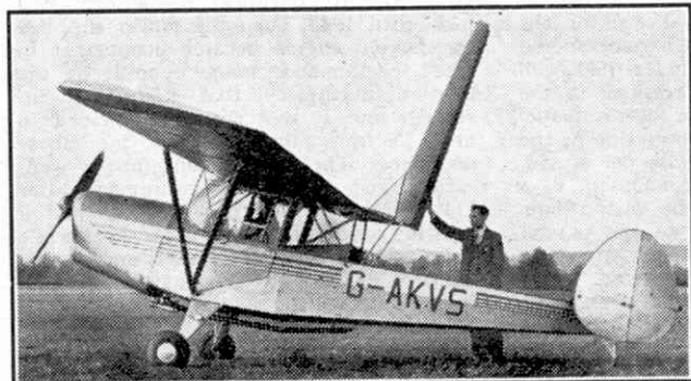
Chrislea "Skyjeep," showing how the top part of the rear fuselage can be raised to permit easy loading of a stretcher or light freight. Photograph by courtesy of Chrislea Aircraft Co. Ltd.
