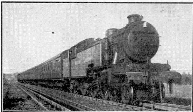
An up train bound for Marylebone on Ruislip Troughs. The engine is L.N.E.R. type 2-6-4 T of Class L1, No. 67714. Photograph by C. R. L. Coles.
