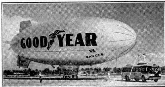
The "Ranger" was operated by the U.S. Navy during the Second World War. On the right is a portable mooring mast.
