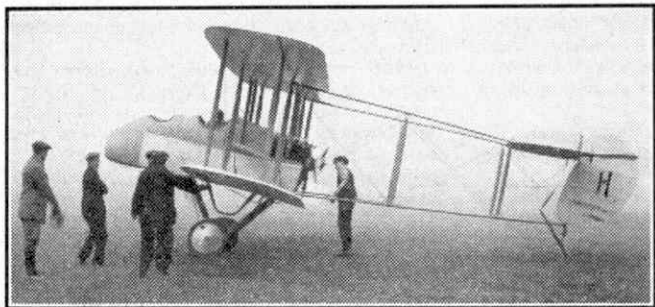
The D.H.1, from which was developed the famous D.H.2 "pusher" fighter of 1916. Photograph "Flight" Copyright.
