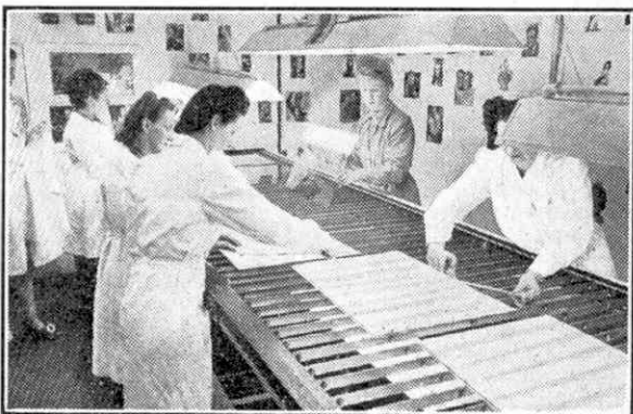
Assembling the constituents of sheets of laminated safety glass and trimming the edges of the vinal interlayer.
