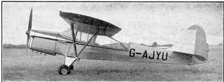
"Auster" Mk. 5D, a new version of the popular Mark 5, which has a "Gipsy Major" engine instead of the usual Lycoming, to overcome the difficulty of obtaining spares for the American engine. Photo. courtesy Auster Aircraft Ltd.
