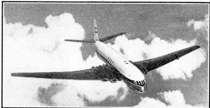
D.H. "Comet," with new B.O.A.C. colour scheme. The white top reduces the cabin temperature in tropical areas. Photograph by courtesy of de Havilland Enterprise.
