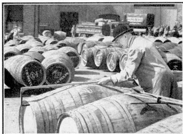
A member of the Landing staff, who do not wear uniform, gauges a cask of wine to assess the duty.
