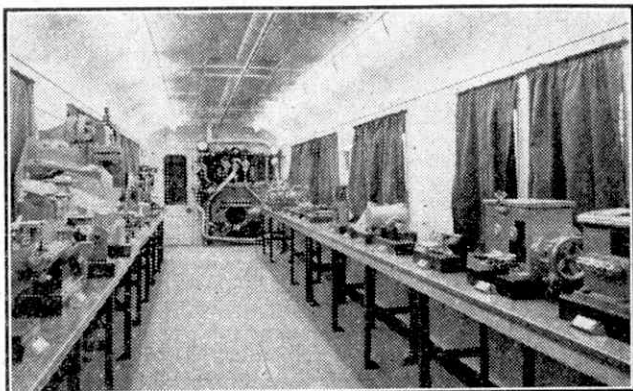
A boiler end with cab fittings is a feature at the far end of this L.M.R. instruction car.
