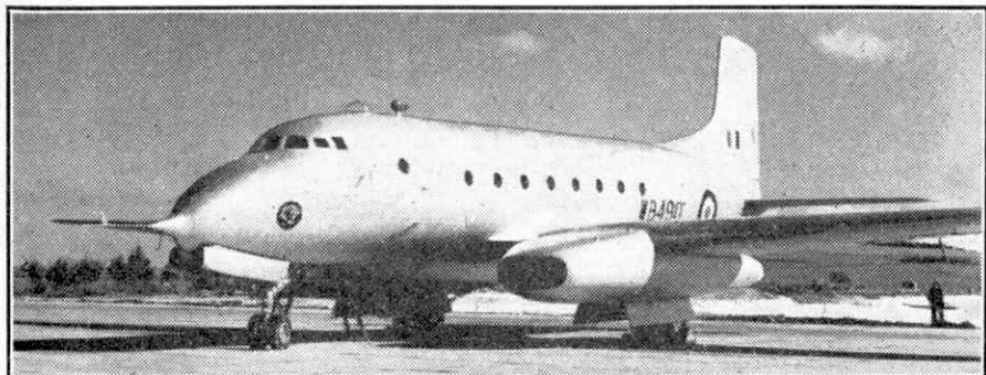
The four-jet Avro "Ashton," designed as a flying laboratory for high-speed, high-altitude flight research. Photograph by courtesy of A. V. Roe and Co. Ltd.
