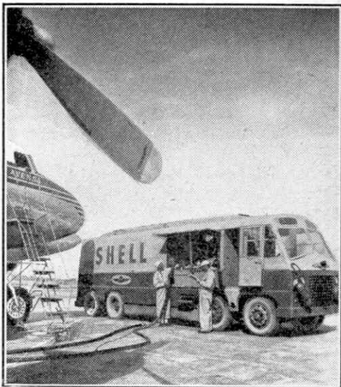
The world's largest aircraft fueller "feeding" a Douglas DC-4 air liner at a Venezuelan airport. This new giant Thompson-Leyland mobile fueller has a capacity of 4,000 Imperial gallons and a maximum delivery rate of 400 gallons a minute. Photograph by courtesy of Shell Petroleum Co. Ltd.
