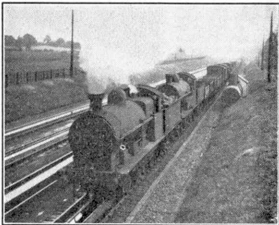
This picture taken some years ago shows one of the familiar ex-L.N.W.R. 0-8-0s at Whitmore troughs. The second engine is a "George the Fifth" 4-4-0 "Widgeon" being hauled to Crewe for scrapping.
