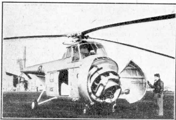
In this view of the Sikorsky S.55 the big "clam-shell" doors at the nose are open, revealing the 600 h.p. Pratt and Whitney engine.
