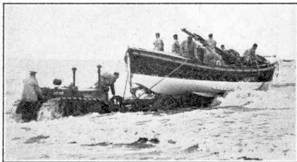
A launch by tractor at Skegness. Photograph by courtesy of "The Skegness News."
