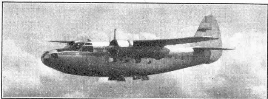
P.54 aerial survey version of the twin-engined Percival "Prince," showing the camera aperture doors open. Photograph by courtesy of Percival Aircraft Ltd.
