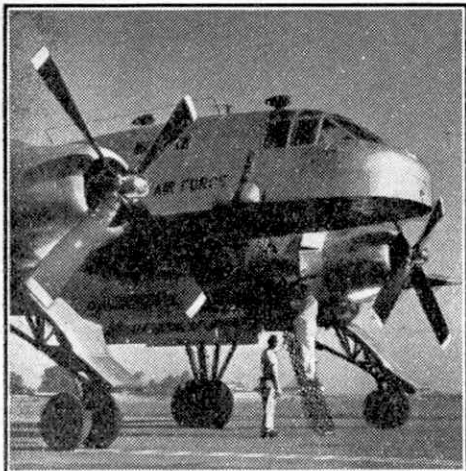
The flight deck of the "Pack Plane" is so high above the ground that the aircrew enter and leave it by means of a collapsible ladder when there is no cargo container under the fuselage. Photograph by courtesy of the Fairchild Aircraft Division, U.S.A.
