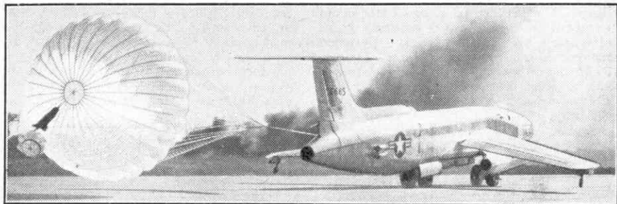
The tail parachute brake of the Martin XB-51 jet bomber reduces the landing speed, enabling the aircraft to touch down on comparatively small airfields. Photograph by courtesy of the Glenn L. Martin Co., U.S.A.
