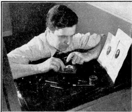
Engraving the steel master die is the first step in the making of a stamp. The engraver cuts the design in soft steel, which is then hardened.
