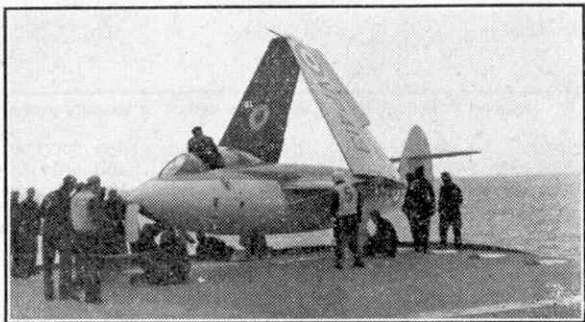
"Sea Hawk" with wings folded, on deck of aircraft carrier. The illustrations on this and the next page are reproduced by courtesy of Hawker Aircraft Ltd.
