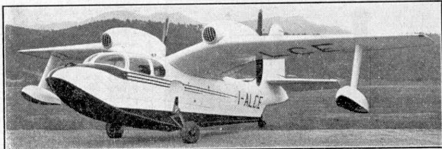
The Piaggio P.136 amphibian, showing the retractable undercarriage and the wing-tip floats. Photograph by courtesy of Piaggio and Company, Geneva.
