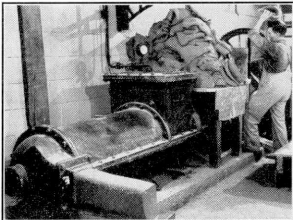
Slabs of clay being thrown into the pug mill, a huge mincing machine from which this raw material for the making of pottery is extruded, ready to be cut into suitable lengths for the potter.
