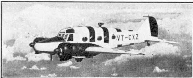
This Anson Mk. 18c is a civil aircrew training aircraft of the Indian Government. A special article on the Anson appears on page 392. Photograph by courtesy of A. V. Roe and Company Ltd.
