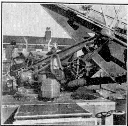
The operating controls of the Morris turntable fire escape ladder. In the centre is the special indicator that automatically stops operation when the ladder has been extended to its safety limit.
