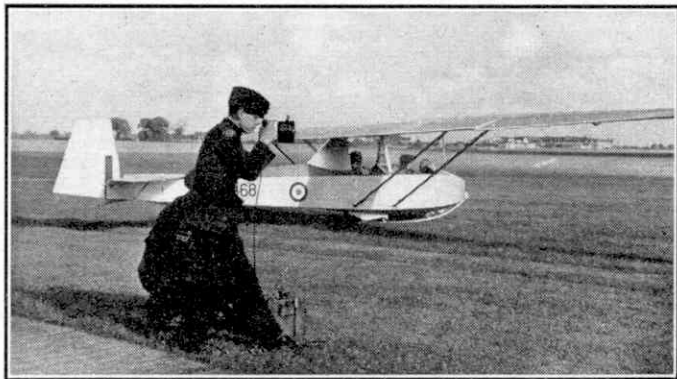
An A.T.C. Cadet signalling the launching winch as the Slingsby Tutor glider prepares to take off. Air Ministry Photograph.
