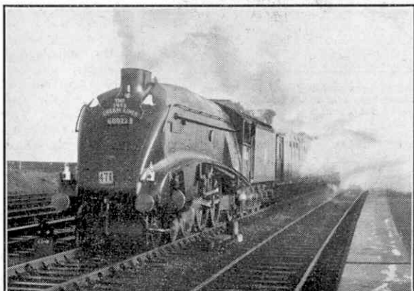
Gresley Pacific "Mallard" displays classification flags as used in American railroad practice to indicate that the train is running as an "extra." The train is the 1952 Dreamliner special referred to in the accompanying notes. British Railways (North Eastern Region) Official Photograph.
