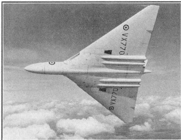
Remarkable underneath view of the giant Avro 698 bomber, showing its delta form. Photograph by courtesy of Hawker Siddeley Group Ltd.
