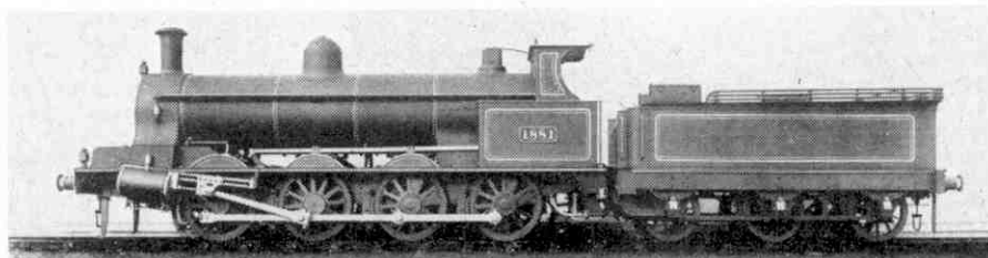
An L.N.W.R. Webb Compound 0-8-0 coal engine with the piano-front casing prominent ahead of the smoke-box. Many of the class were converted to superheated simple engines. British Railways Photograph.
