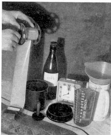
Loading a film in an apron type tank.
