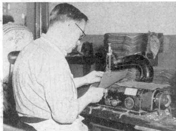
The craftsman at work here is skivering leather, that is paring it to half thickness at the edges to allow for turning these over when making up into binding cases for diaries.
