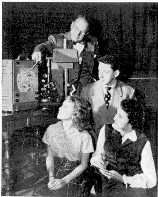
A microscope with the television apparatus that shows an enlarged picture of the object on a screen that can be seen easily by many onlookers at once. We are indebted to the Radio Corporation of America for this illustration and for the information in the accompanying article.
