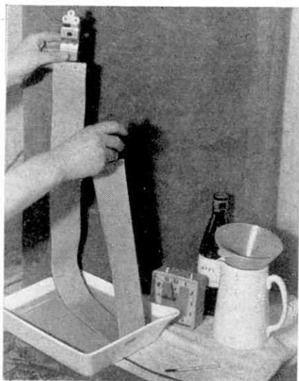
Developing a film in a dish by see-saw methods. The illustrations to this article are from photographs by the author.
