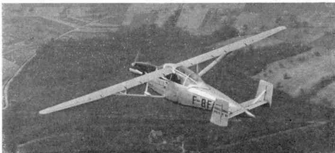
The French Hurel Dubois H.D.10 research aircraft, which has exceptionally long and narrow wings.
