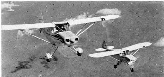
Piper Pacer 135 and Tri-Pacer 135 light aircraft. "Tri" indicates tricycle undercarriage.
