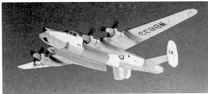
Avro Shackleton with bomb doors open and radar extended. Photograph by courtesy of A. V. Roe and Co. Ltd.
