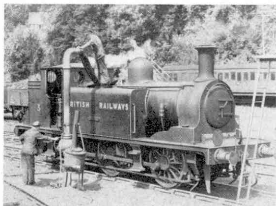
Here is 0-6-0T Ryde, No. W3 of the Isle of Wight section of British Railways Southern Region, taking water. This effective view is from a photograph by R. Russell.
