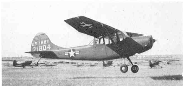
Cessna XL-19B Bird Dog, the world's first propeller-turbine powered light aircraft, taking off on its maiden flight at Wichita, Kansas. Photograph by courtesy of Boeing Airplane Company, U.S.A.
