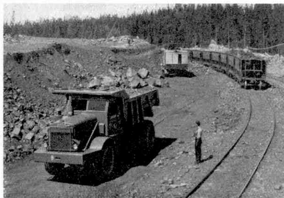
Lorries bring ilmenite to the siding where the ore is loaded into railway trucks, for despatch to the smelting plant at Sorel.
