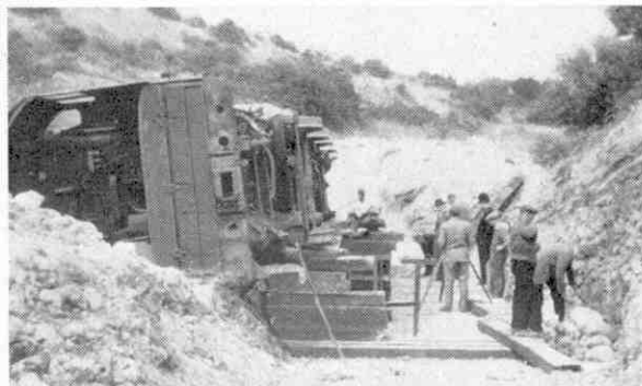
First steps in recovering this derailed Lord Nelson class locomotive were to dig a pit alongside and to lash rails to its wheels before rolling it upright.
