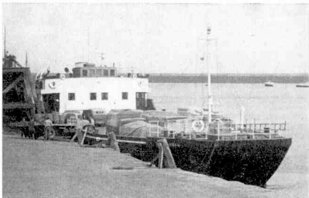
Glenfinnan alongside the landing stage at Granton. This vessel is one of the converted Landing Craft Tanks that are used on the Granton-Burntisland ferry.
