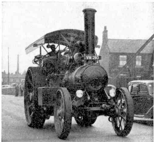
Atlas, a Fowler road engine completed in April 1928. It is equipped with a dismountable jib crane, the winding drum for which is seen on the off side, just forward of the top of the rear wheel. Photograph by courtesy of S. Mustill, Huyton, the present owner of Atlas.
