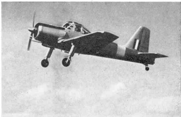
Percival P.56 Provost trainer, powered by 550 h.p. Alvis Leonides engine, now in production for the Royal Air Force.
