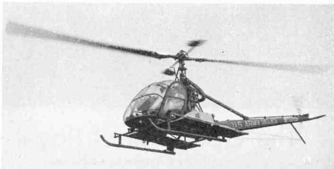
U.S. Army H-23B helicopter with external heated litters, as used on casualty evacuation service in Korea. Photograph by courtesy of Hiller Helicopters, U.S.A.
