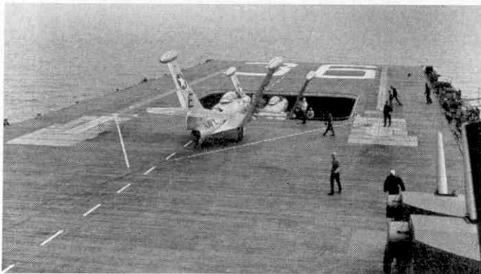
Panther aircraft going down the lift to the below-deck hangars. At one stage they were landing and going below at 30 sec. intervals. Photograph by courtesy of Hawker Siddeley Group Ltd.
