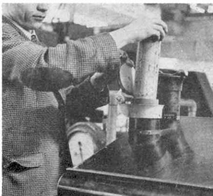
A container carrying a sample of steel is inserted in the tube in which it is carried to the laboratory for analysis.
