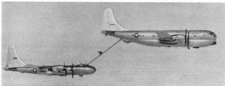
A pair of Boeing team-mates "hook up" high above the clouds as a KC-97 Stratofreighter provides a B-50 Superfortress with a new load of fuel. Photograph by courtesy of the Boeing Airplane Company, U.S.A.
