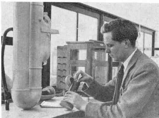
The report on a sample of steel is returned to the melting shop by tube. The illustrations to this article are reproduced by courtesy of the Steel Company of Wales Ltd.
