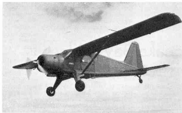
New version of the Canadian-built DHC-2 Beaver light transport, powered by a 550 h.p. Alvis Leonides engine. Photograph by courtesy of de Havilland Enterprise.
