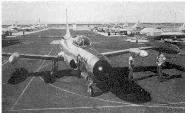
Lockheed F-94C Starfire jet fighter with pod containing 12 rockets mounted on the leading edge of each wing, as described on this page. Photograph by courtesy of Lockheed Aircraft Corp., U.S.A.
