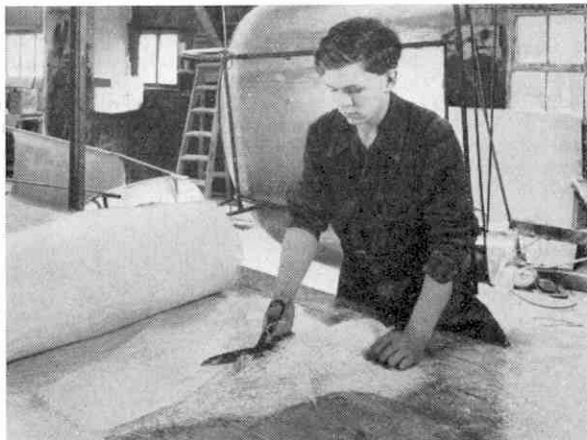
Here the glass fibre mat is being cut out to pattern in readiness for building up into a car body.
