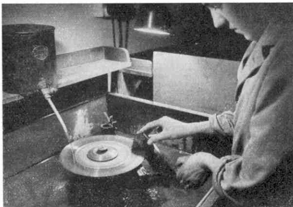
A meteorite found at Beddgelert in January 1950 is here seen being cut into two pieces by a revolving steel plate that has diamond dust forced into the nicks on its edges.
