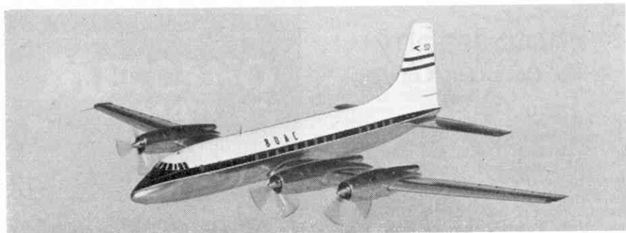
Latest picture of the prototype Bristol Britannia turboprop air liner, showing the new jet exhausts. Photograph by courtesy of The Bristol Aeroplane Co. Ltd.
