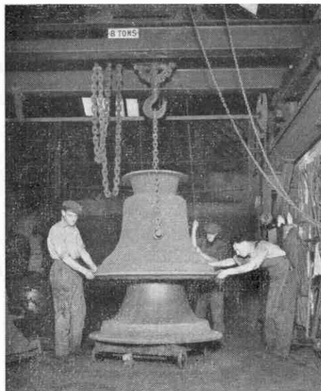
Building up the mould in which a bell is to be cast. The two parts are moulded separately and here the outer mould is seen being lowered over the inner one.
