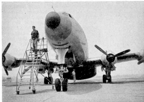
Ground view of the RC-121C. The 8ft. high hump on the back, the huge bulge underneath and the elongated nose house radar antennae.
