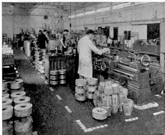
Wellworthy Al-fin cylinder barrels being machined.
