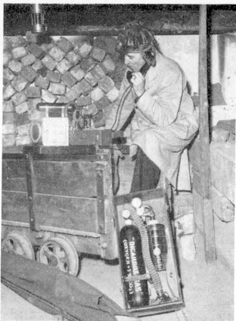
The Senior Instructor of the Coatbridge Mines Rescue Team telephones men dealing with a mock fire during a demonstration. In front of him is a "humane" cage, with a canary in it.
