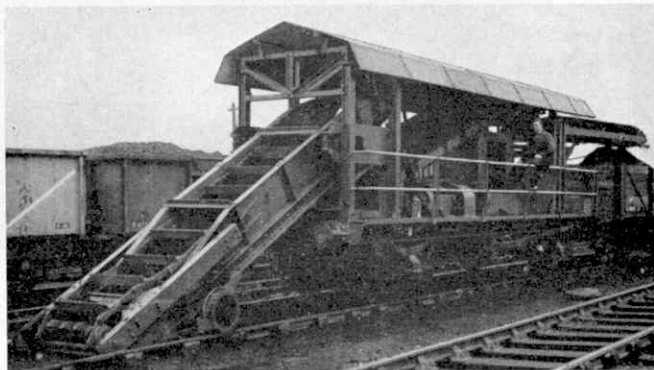
A diesel-driven machine used to clear coal from sidings. Photograph by J. Balmond, Birmingham.
