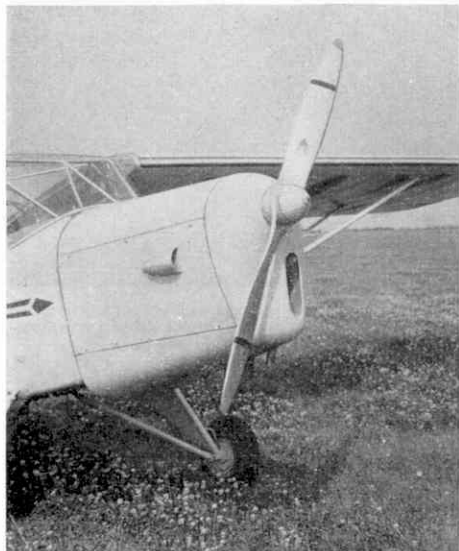
A typical Fairey-Reed metal propeller on an Auster lightplane. These propellers are made from a single piece of metal, machined and twisted to the correct shape.
