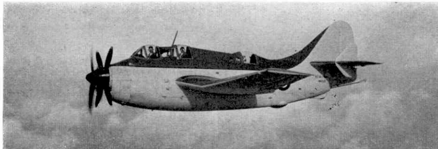
One of the Fairey Gannet's two contra-rotating, co-axial propellers feathered in flight with the aircraft cruising on a single engine to save fuel. On some aircraft, like the Westland Wyvern, one engine drives two contra-rotating propellers through gearing. The Gannet has two engines, each driving one propeller.
