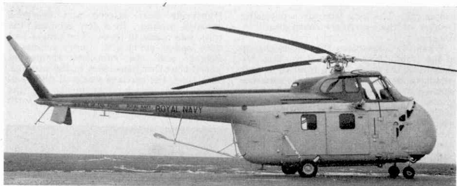
Westland Whirlwind helicopter of the Fleet Air Arm, fitted with hook under the tail-boom as part of special equipment for mine-sweeping duties.
