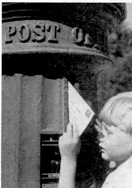
Have you ever seen a pillar box with a vertical slot? This one, photographed by F. Read, is at Mudeford, near Christchurch, Hants. The idea of the design was that a sack to receive letters could be hooked up behind the slot.
