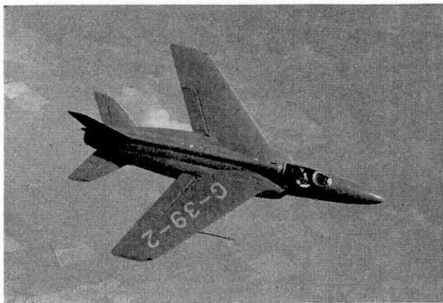
The Folland Gnat lightweight fighter, showing the inboard ailerons with which it is equipped. Photograph by Cyril Peckham.
