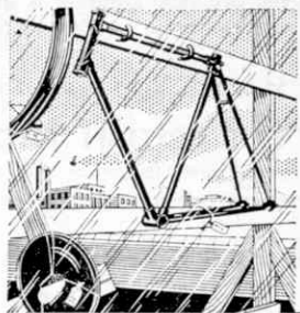
All the enamelled Triumph parts on the roof of the factory where they remained for over a year!
