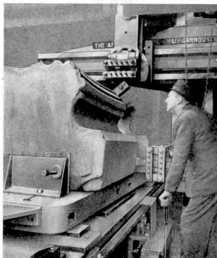
A planing machine that is used for shaping large stone blocks for Liverpool Cathedral.
