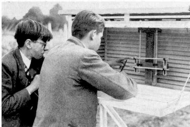
Boys of the school reading instruments inside the weather station Stevenson Screen.
