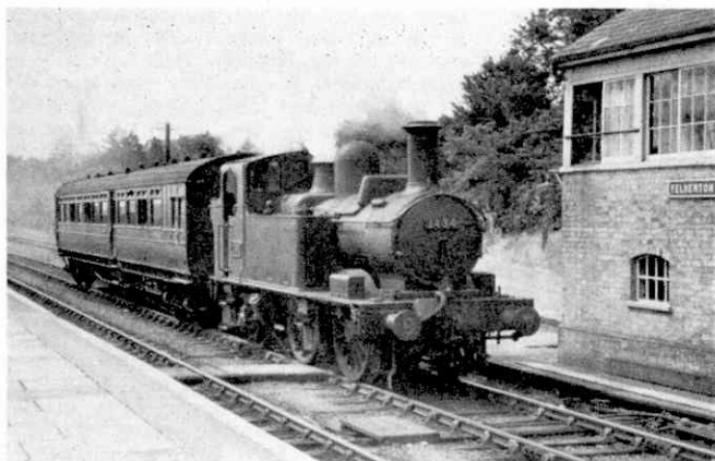
A pleasing view of a Western Region motor train or push-pull unit approaching Yelverton on its way to Tavistock from Plymouth, Road North. The engine is 0-4-2T No. 1434. Photograph by R. E. Vincent.
