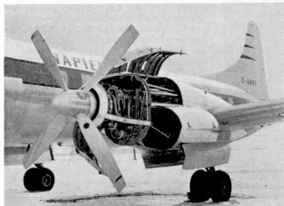
This view of the port Eland turboprop in the Napier-owned Convair-340 shows the ease of access to the engines.
