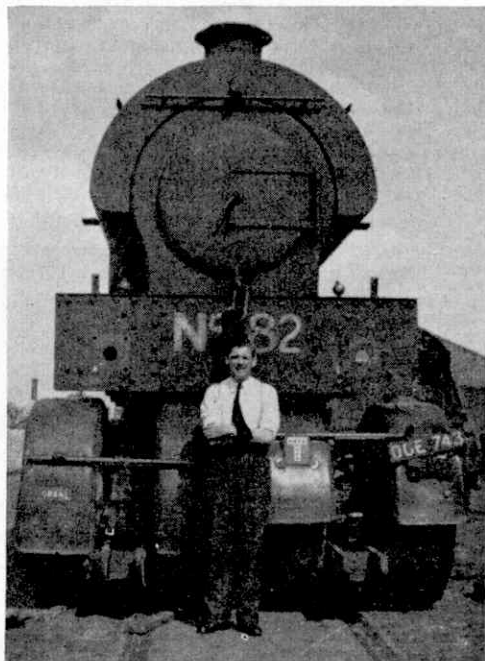
What is this? A new type of locomotive? A clue to the answer is given by the road registration on the right and the T sign to the left of it. The photograph is that of a steam locomotive on a trailer for road transport, and was taken by S. Harvey, London E.11.
