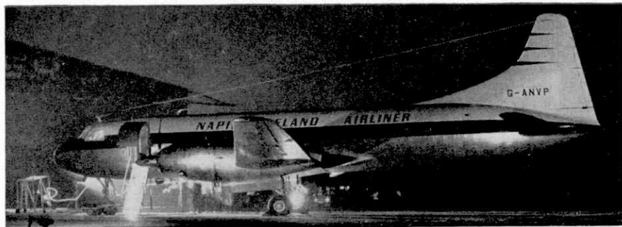
A night photograph of the Convair-340 bought by Messrs. D. Napier & Son, showing it equipped with Napier Eland turboprops in place of its original Pratt and Whitney piston engines.
