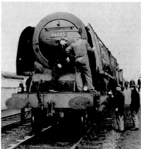
Preparing L.M.R. No. 46225 "Duchess of Gloucester" in March last at Skipton before a special run to Carlisle with dynamometer car and mobile test units. Photograph by W. Hubert Foster.
