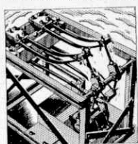
THE FRONT FORK TEST Ten million jolts worth of vibration in this machine tested the enduring quality of the Triumph front fork, & proved its great strength
