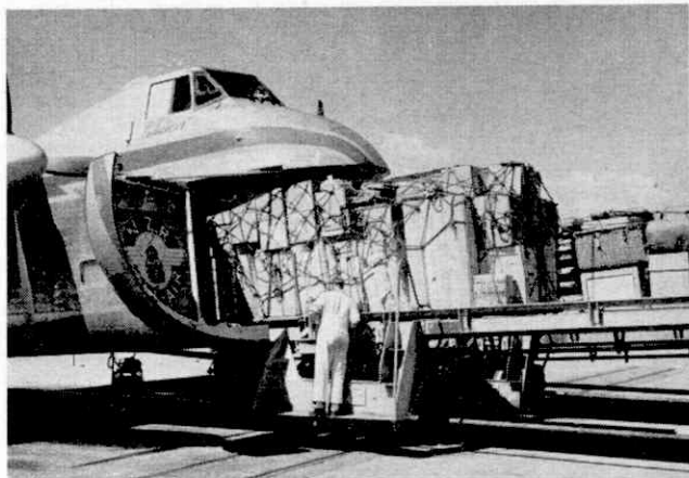
Mixed general freight being loaded "en bloc" into an aircraft of Straits Air Freight Express, New Zealand.
