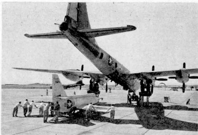
The X-2 on its carriage being pushed under the fuselage of the "mother-plane" which has been raised to receive it. The illustrations to this article are by courtesy of the Bell Aircraft Corporation, U.S.A.
