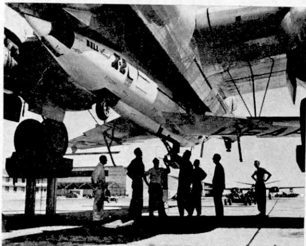
In this picture the X-2 is shown attached to the underside of the fuselage of the parent aircraft.
