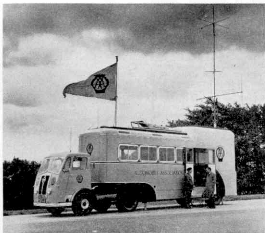
The radio control network of the Automobile Association now incorporates two of these mobile headquarters, known as Jumbos.
