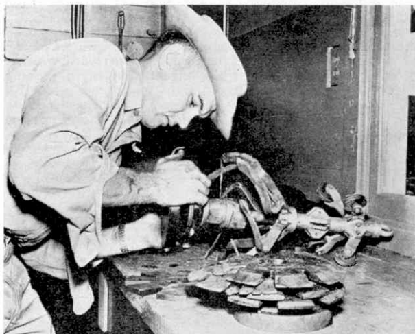
Replacing rubber discs on a go-devil at a pump station repair shop. In the foreground are notched discs worn by use in a pipeline of varying diameter.
