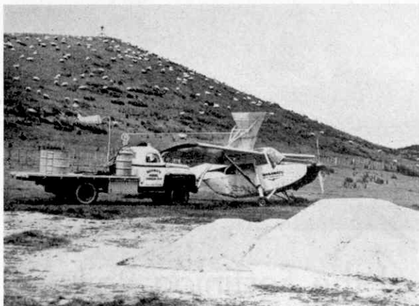
The Edgar Percival E.P.9 agricultural aircraft was designed primarily for farm work in New Zealand. Here one of these machines, bought by the Manawatu Aerial Topdressing Co. Ltd., is being loaded with superphosphate during a demonstration at Christchurch, N.Z.
