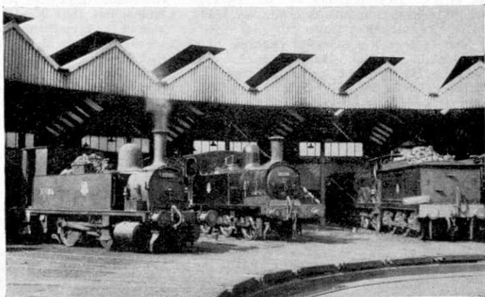
At Guildford, in the Southern Region of British Railways, tracks radiate from the turntable to serve an engine shed of the roundhouse type. Photograph by S. Creer.
