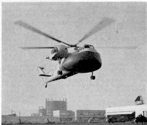
The latest version of the American Sikorsky HR2S-1 helicopter has a large radar scanner that is housed in the conspicuous "blister" seen under the cockpit.
