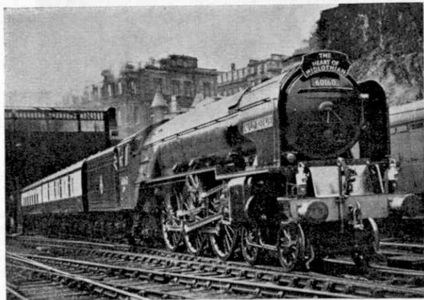
The "Heart of Midlothian" leaves Waverley for the South in charge of the impressive A1 Pacific No. 60160, "Auld Reekie," an appropriate revival of the title of an N.B. Atlantic.
